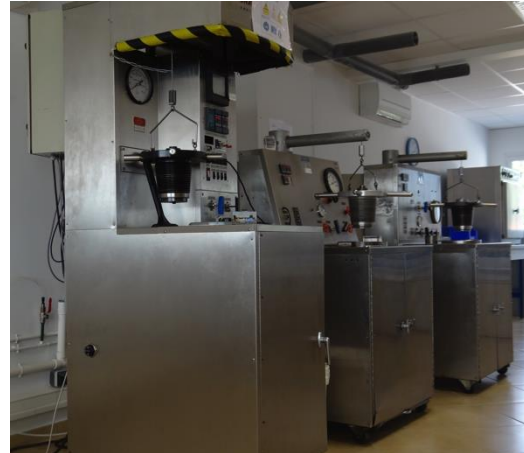
CURISTEC ISO9001 certified laboratory with HTHP cement consistometers
