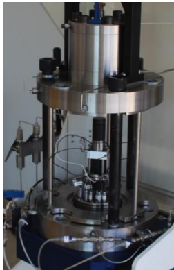
Triaxial load cell to evaluate cement mechanical properties
